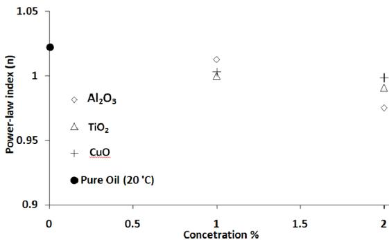
Figure 6. Effects of nanoparticle concentration on the power-law index
