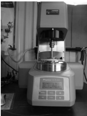
Figure 2. Anton paar rheometer
