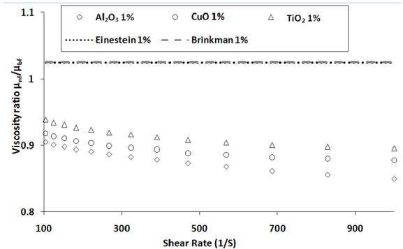
Figure 8. Effects of nanoparticle addition and shear rate on the viscosity of the nanofluids (at 1 wt.% concentration)
