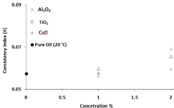
Figure 7. Effects of nanoparticle concentration on the consistency index
