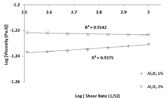
Figure 5. Variation of viscosity of the  $Al_2O_3$ -oil at 1 and 2 wt.%
