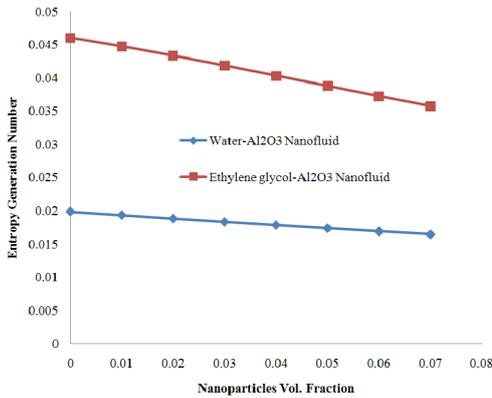
Fig. 6. Comparison between the entropy generation numbers of the water-Al<sub>2</sub>O<sub>3</sub> with ethylene glycol-Al<sub>2</sub>O<sub>3</sub> at the same condition.
