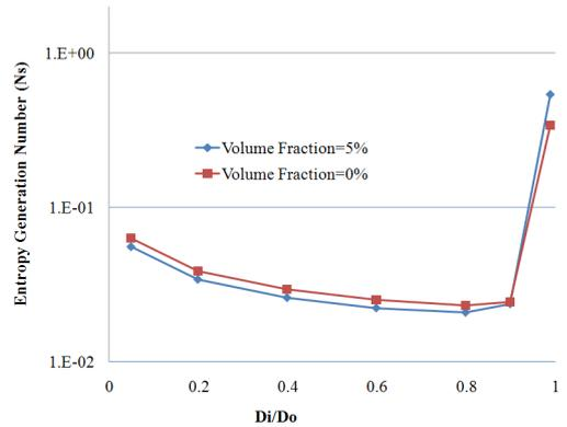
Fig.8. Variations of the entropy generation number ( $T_0 \dot{S}_{gen} / \dot{Q}$ ) with diameter ratio for length ratio of 500.
