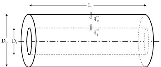
Figure 1. Geometric configuration of the concentric tube annulus
