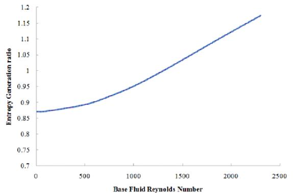
Fig. 9. Dependency of the irreversibility to the base fluid flow Reynolds number for:  $D_i/D_o=0.8$ ,  $L_e/D_h=1000$ ,  $\phi=5\%$  and  $Q^*=197.5$  Watt
