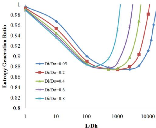
Fig.7. effects of diameter ratio on the entropy generation ratio of the water-Al<sub>2</sub>O<sub>3</sub> nanofluid flow.
