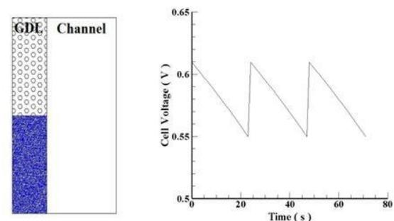
Fig. 5. Voltage drop curve with GDL flooding assumption
