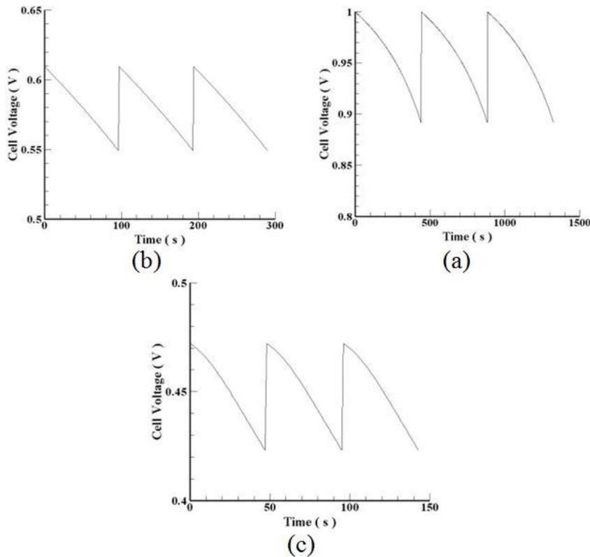
Fig. 7. Voltage drop in different current densities a)  $0.5 \text{ A/cm}^2$ , b)  $1 \text{ A/cm}^2$  and c)  $1.5 \text{ A/cm}^2$
