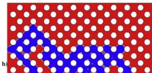
Fig. 2. a) Geometry of the model, b) Water distribution in GDL [10]
