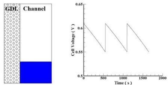
Fig. 4. Voltage drop curve with channel flooding assumption
