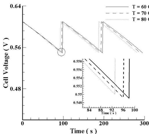
Fig. 8. Effect of temperature on voltage drop curves
