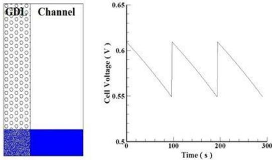
Fig. 6. Voltage drop curve with GDL-channel flooding assumption
