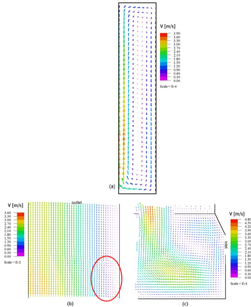
Fig.5. Distribution of velocity vectors of water and gas in case a - without vent hood and flue baffles (a) water tank (b) fired tube, and (c) lower space with intake window. The return flow of cold air with high density is clearer in Figure (5-b).
